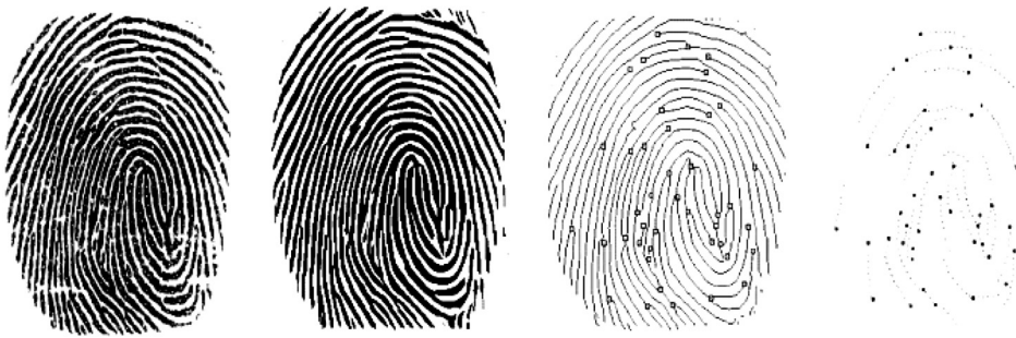
FIG 6. – Processing steps of the UPM-minutiae based verification system.
