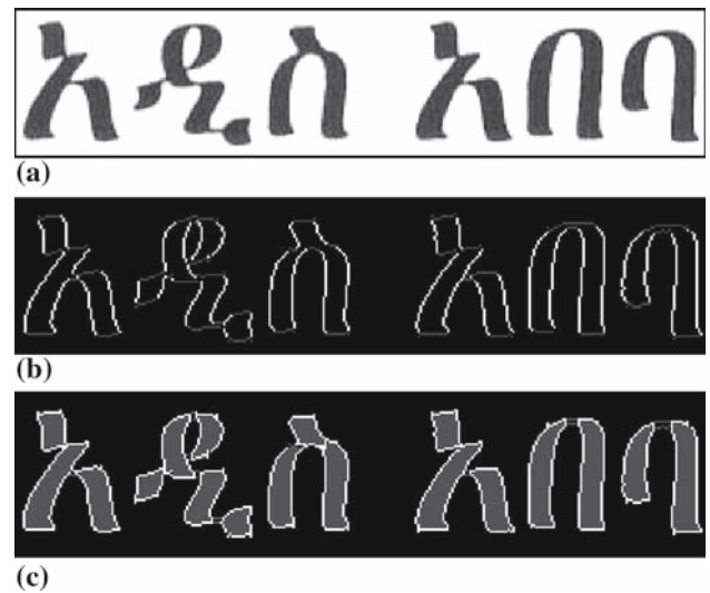
Fig. 7 a Ethiopic text, b primitive lines shown as white lines, and connectors shown as the gray lines, c extracted primitive structures
