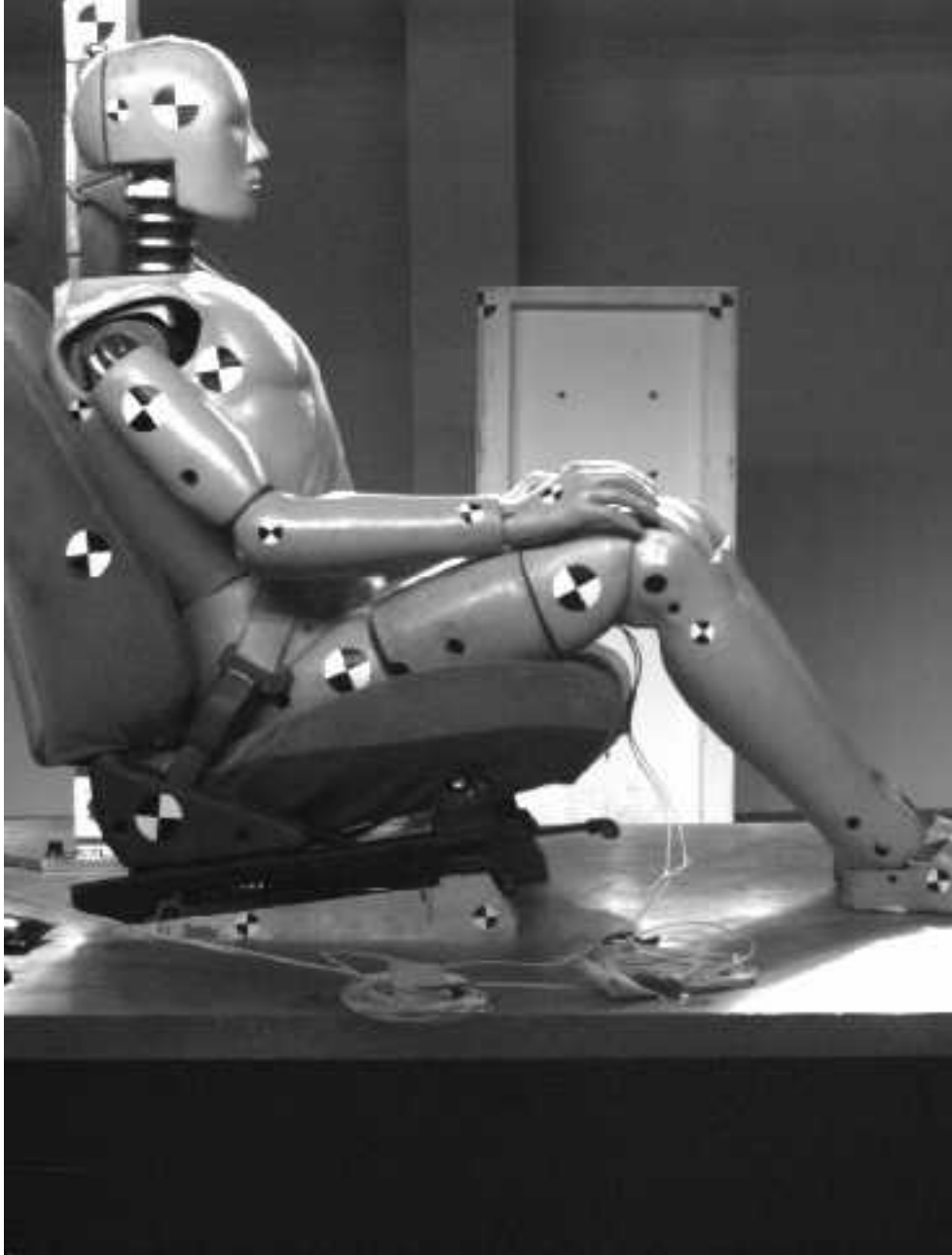
Figure 1: The first frame of an image sequence in which cross markers should be tracked.
