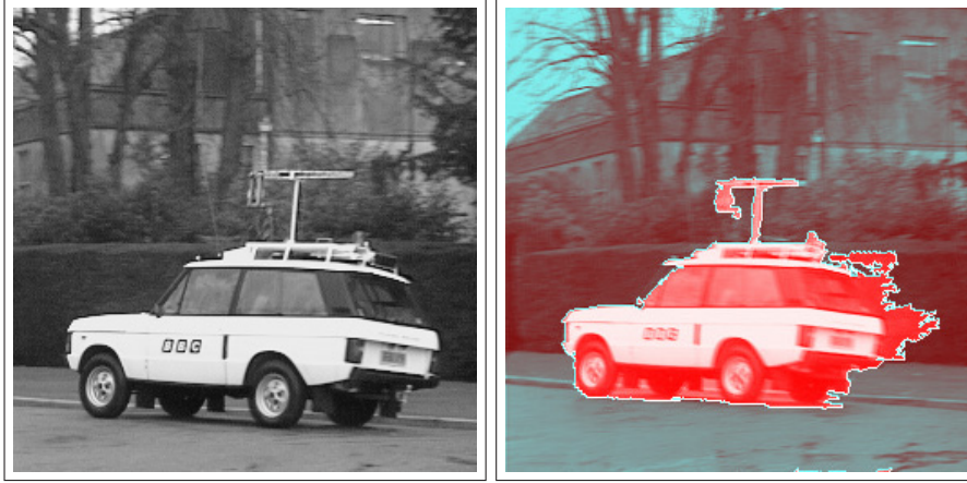
Fig. 12.5. Affine motion is estimated from 5 images ( right ) [61], using the eigenvectors of (12.92). One of the original frames is shown on the left . On the right , the red car region, and the cyan-labeled background region have different affine motion parameters which were found automatically
