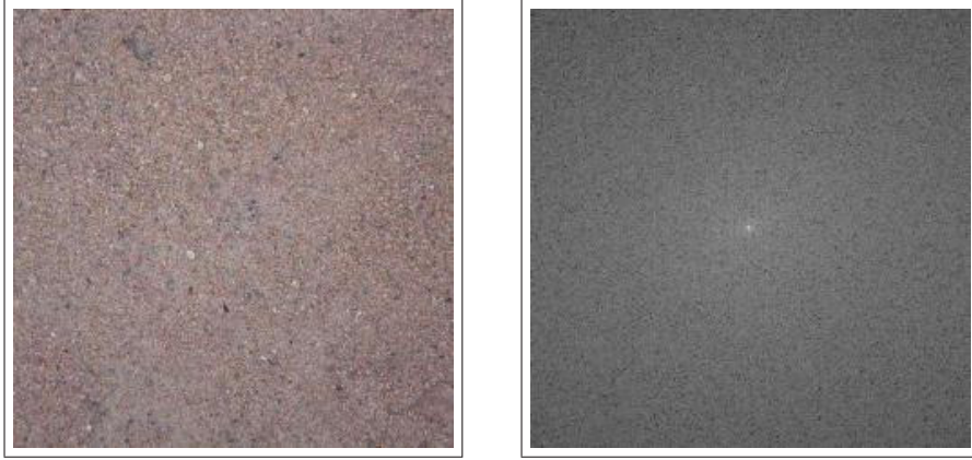
Fig. 10.13. Left: a real image that is not linearly symmetric. It shows a close up view of sand. Right: The Fourier transform magnitude of a neighborhood in the central part of the original image. Notice that the power is isotropic i.e., far from being concentrated to a line
