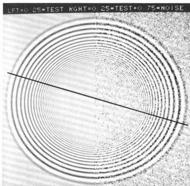
Figure 2: The test image used in the experiments. The straight line is the line along which the profiles of results are presented at the proceeding figures.
