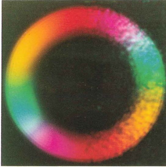
Figure 14: Indication of linear symmetry, with the brightness \lambda_1 - \lambda_0 and the hue indicating orientation. It is obtained by filtering Figure 13 with a 21x21 filter.
