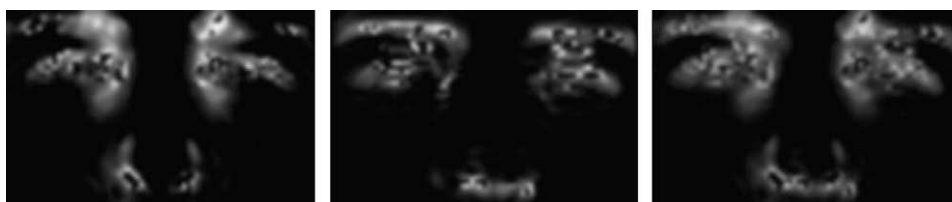
Fig. 6. Example face center template for OF pattern matching: horizontal OFL (left); vertical OFL (middle); magnitude of combined OFL (right) (Gabor-filtering used [5]).
