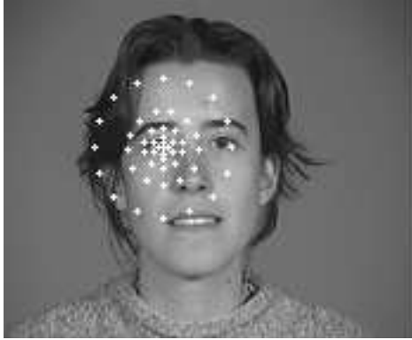
Figure 3: The extended model of a facial landmark is obtained by centring the retina on that landmark in the images of the training set.
