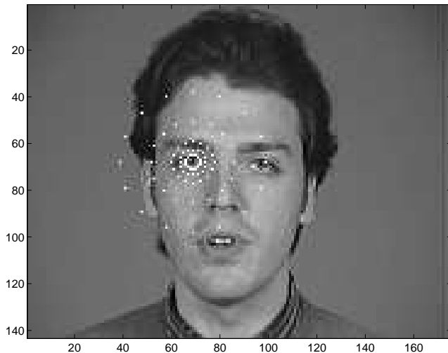
Figure 2: The retinal sampling grid placed on a person’s right eye for model creation.
